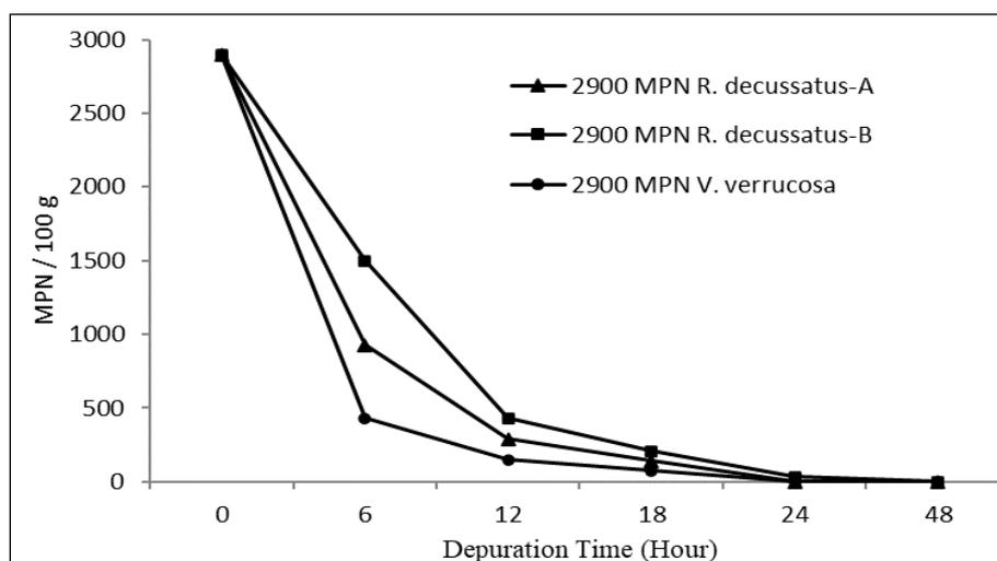
Figure 2. Depuration times of *R. decussatus* (batch-A and B) and *V. verrucosa* contaminated with *E. coli* at 2900 MPN/100g representing class B production areas.
